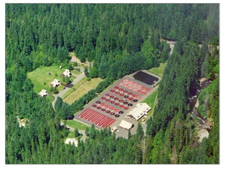
Marion Forks Hatchery has 34 stacks of heath stack vertical incubators. Because of the hatcherv's cold water supply, it is equipped with a water heating system that enables the operators to increase growth rates in attempts to meet target sizes. Marion Forks Hatchery is equipped with 12 Canadian-style troughs and 48 circular ponds. There are no spawning facilities at Marion Forks: all spawning occurs at Minto Pond. The ODFW
