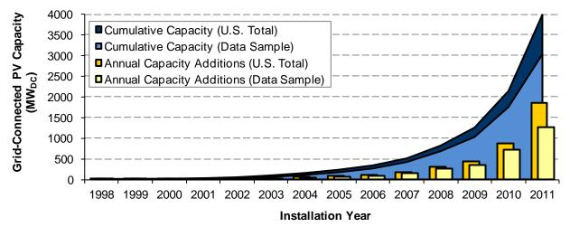
Data source for U.S. total grid-connected PV capacity additions: Sherwood (2012) Figure 1. Data Sample Compared to Total U.S. Grid-Connected PV Capacity
