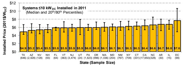
Notes: Median installed prices are shown only if 15 or more observations were available for a given state. Figure 16. Installed Price of Residential & Commercial PV Systems by State (≤10 kW Systems)
