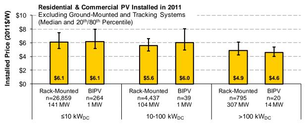
Figure 22. Installed Price of BIPV vs. Rack-Mounted PV Systems
