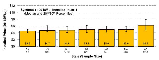
Notes: Median installed prices are shown only if 15 or more observations were available for a given state. Figure 18. Installed Price of Residential & Commercial PV Systems by State (>100 kW Systems)
