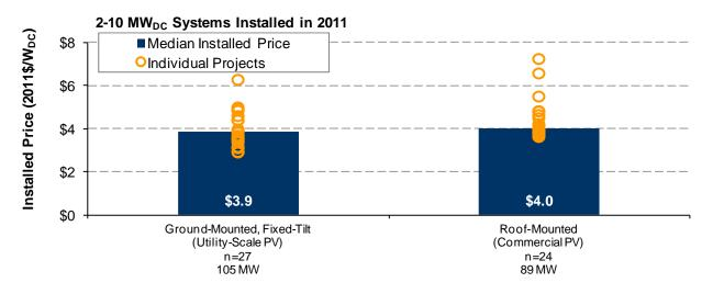
Figure 31. Installed Price of Small Utility-Scale PV vs. Similarly Sized Commercial Rooftop PV
