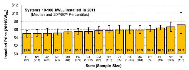
*Notes: Median installed prices are shown only if 15 or more observations were available for a given state.* **Figure 17. Installed Price of Residential & Commercial PV Systems by State (10-100 kW Systems)**
