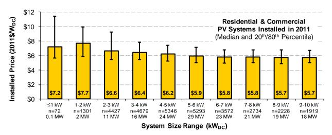
Figure 15. Installed Price of Residential & Commercial PV According to System Size (≤10 kW)
