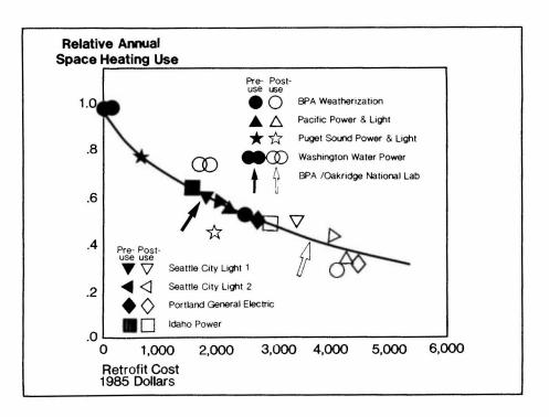
**Figure 5-2** Comparison of Regional Thermal Integrity Curve Estimated Cost and Savings Compared to Observed Bill Changes in Existing Utility Weatherization Programs
