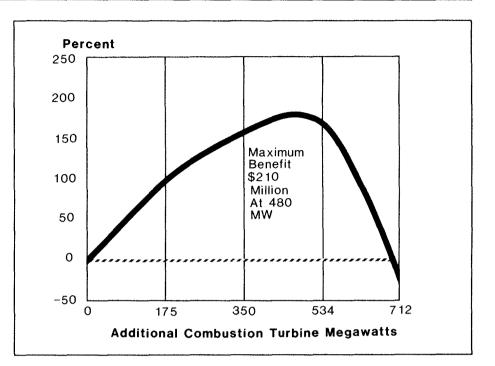
Figure 7-15 Net Benefits of Combustion Turbines vs. Coal (Based on Comparison to Coal Plants)
