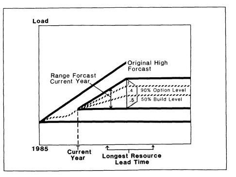
Figure 8-6 Option and Build Level
