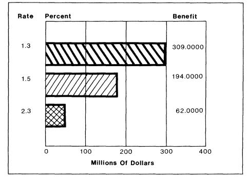
Figure 7-18 Sensitivity to Fuel Escalation Rate (At 534 Megawatts of Additional Turbine Energy)
